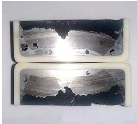
Figure 7: Sample of \text{AlSi}_{12} powder, heated up to 800^\circ\text{C} , in alumina crucible
