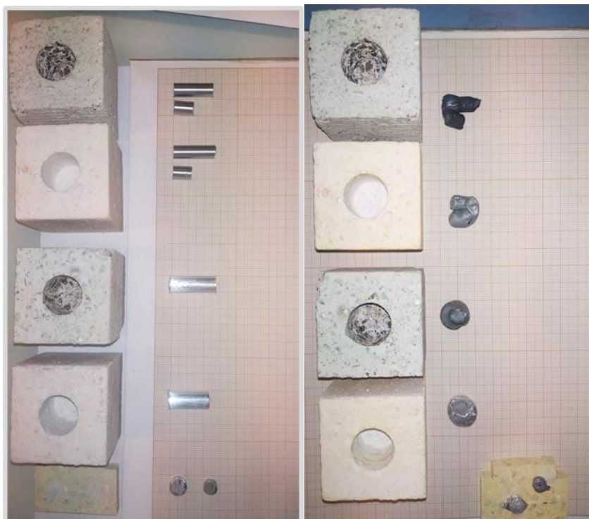
Immersion test Al – AlSi 12 – 700°C – 168h isothermal
