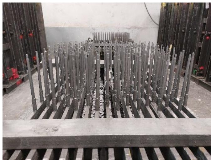
Figure 2: Mold with pins to make the holes
